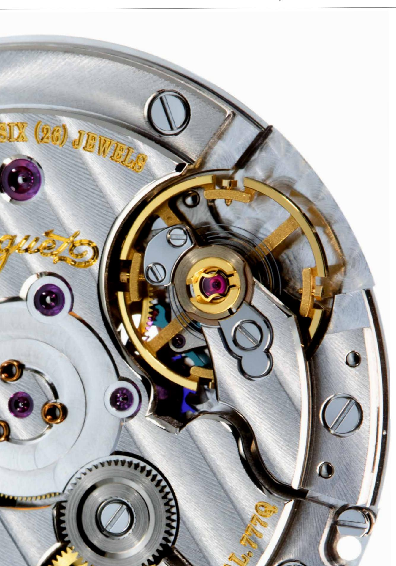
The balance assembly: in total comprising of the balance wheel, four regulating screws, safety roller and impulse jewel (hidden), incabloc shock protection, stud, stud holder, cover plate and screws, balance cock with end-piece securing plate and screw.
